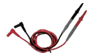
T3002 Probe: Length 120mm, Tip Φ2mm Plug: Φ4mm Cross Plug, right angle type Wire: 22AWG, red/black Length: 800mm Safety Class: EN61010-031, 1000V CATII, MAX 10A
