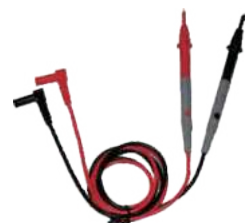
T3001 Probe: Length 130mm, Tip Φ2mm Plug: Φ4mm Cross Plug, right angle type Wire: 20AWG, red/black Length: 1000mm Safety Class: EN61010-031, 1000V CATIII/600V CATIV, MAX 10A
