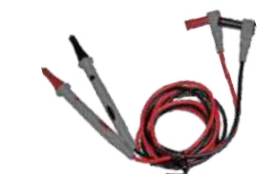
T3006 Probe: Length 130mm, Tip Φ4mm Banana Plug: Φ4mm Banana Plug, right angle type Wire: 18AWG, red/black Length: 1200mm Safety Class: EN61010-031, 1000V CATIII/600V CATIV, MAX 10A
