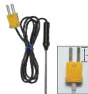
P3409A/B K Type Thermocouple Range: -50~600°C (-58°F~1112°F) Length: 1000mm Type A: Plug Length 12mm, Type B: Plug Length 16mm
